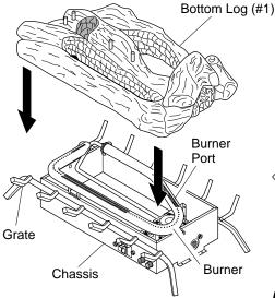
Figure 17 - Installing Bottom Log (#1)
